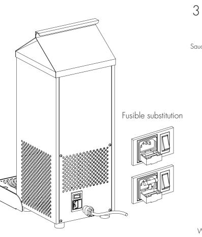
Connect Bricco to the electrical grid through the cable supplied in the packing to pay attention on the feed required from the machine.
